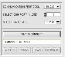
It is now possible to set the baudrate for data transfer through the RS232 interface.
